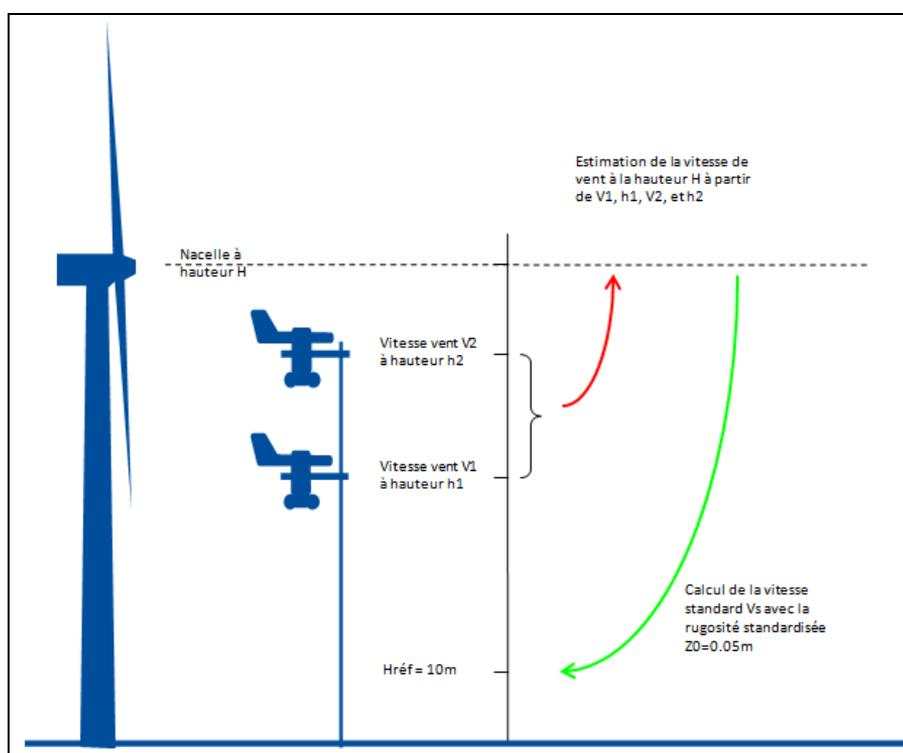
$$V_s = \frac{\ln(10/0.05)}{\ln(H/0.05)} \cdot \left[ V_1 + (V_2 - V_1) \cdot \left( \frac{\ln(H/h_1)}{\ln(h_2/h_1)} \right) \right]$$
